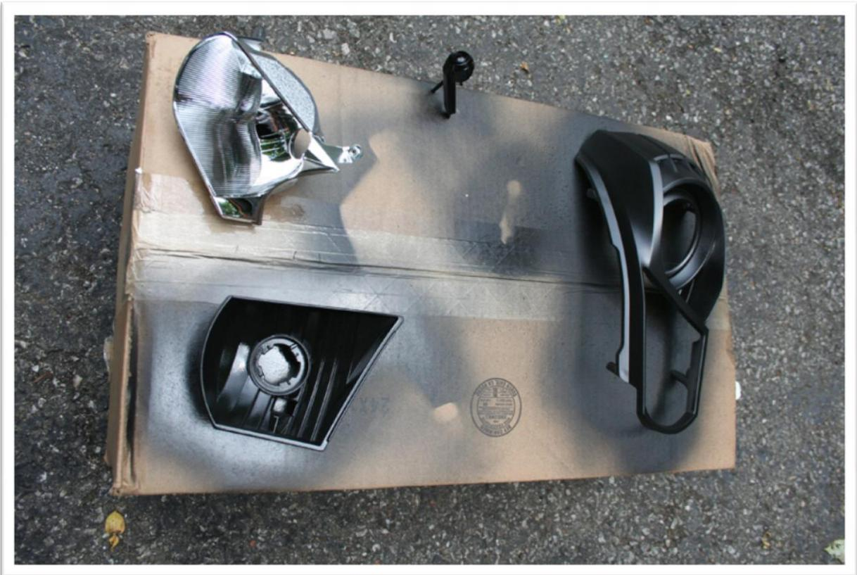
The following are photos of my progress in painting each. This spanned over a 2 hour period and I applied 3 coats of the Plastidip to each, one coat of Nightshades to the reflector and the clear plastic housing to the parking light.
