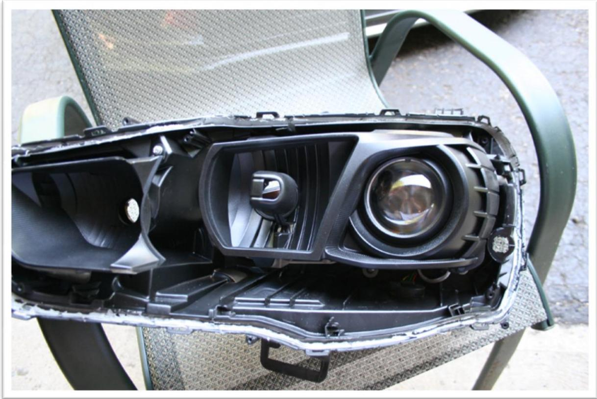
Here the main black tray is inserted over top and screwed down securely.
