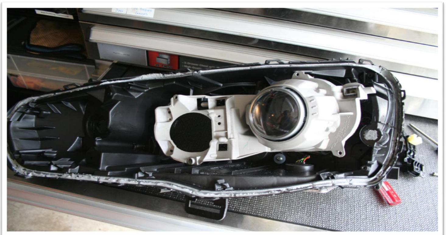
The toughest piece to remove is the large shroud that surrounds the projector. This can be removed by locating these two bolts on the back of the headlight. Use the 10mm socket to back these out of the areas they are screwed into. Once they are backed out (they do NOT come out of the unit), give the chrome housing a small tug to remove it from the metal nub - this is the headlight leveling mechanism.
